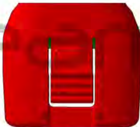
Figure 1: Crack Inspection Area (Green: Allowed Area - Red: Failed Area)
